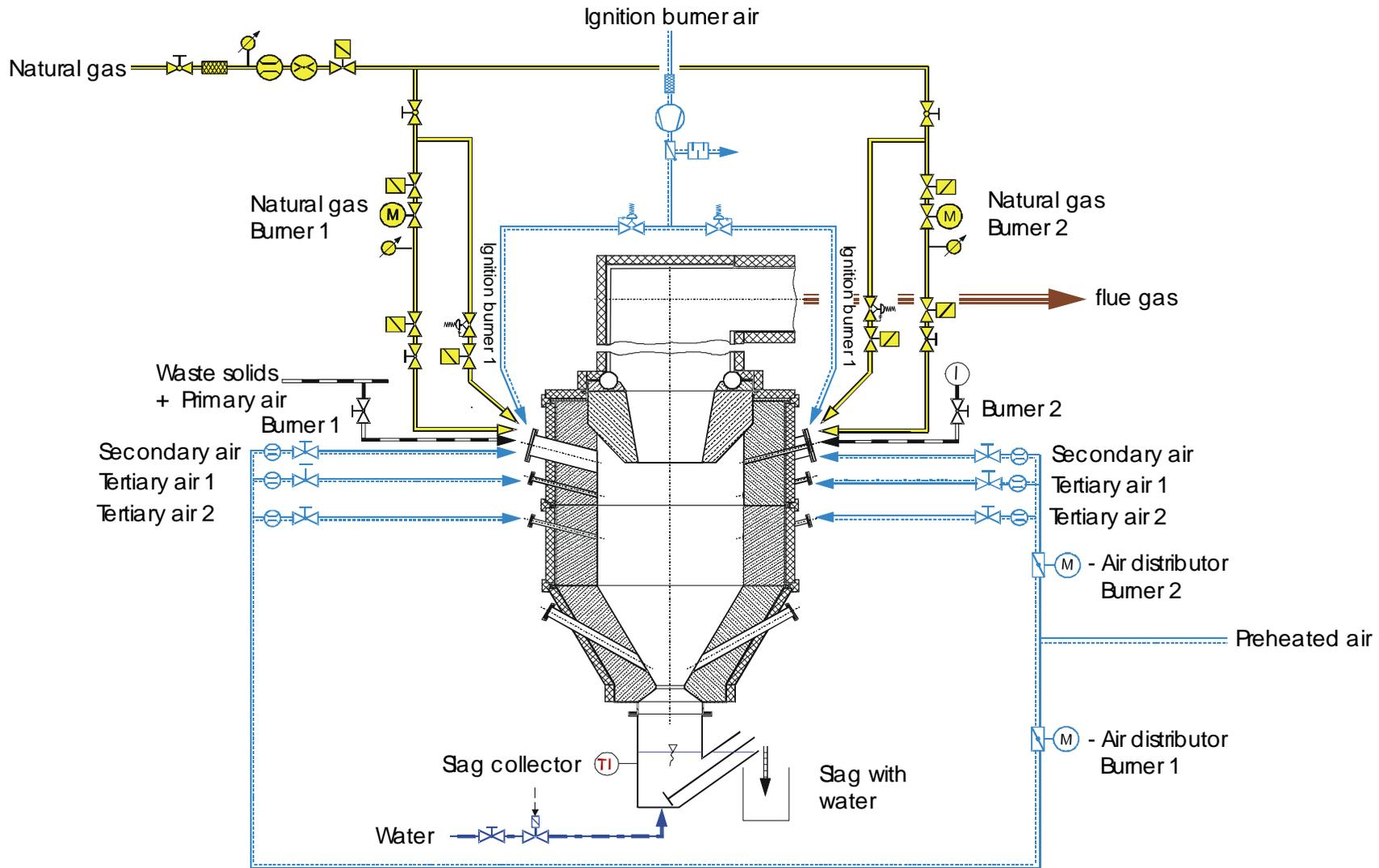
Figure 2: Cyclone slag-tap furnace for thermal utilization of ash-rich waste
