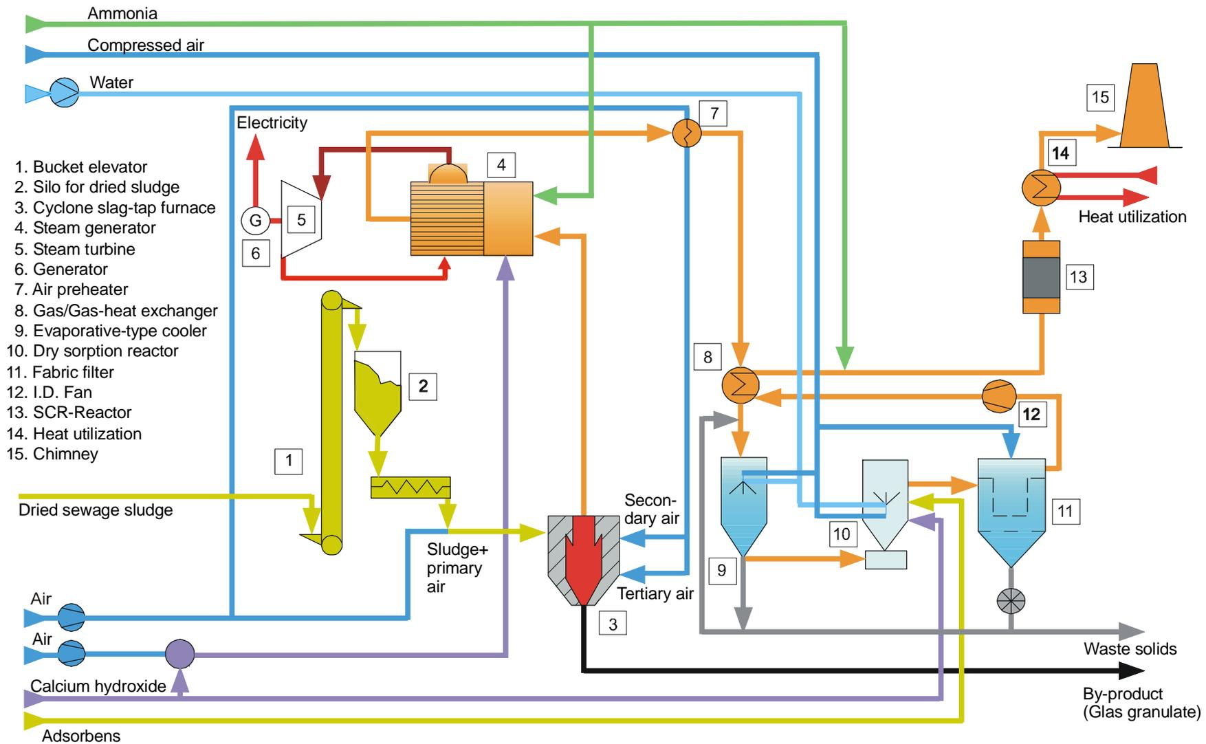
Figure 1: Schematic flow diagram of a thermal utilization plant for ash-rich wastes
